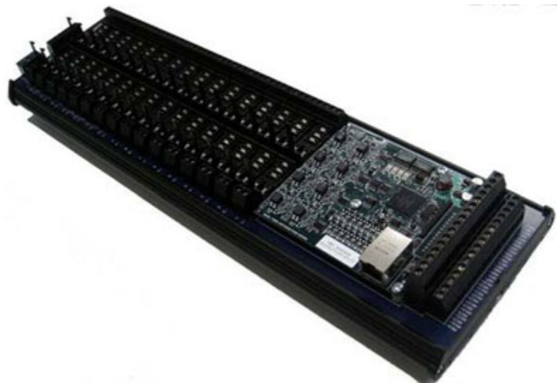
Figure 1 — Freescale Coldfire Processor integrated with CoDeSys on a din rail mounted chassis with 16 Discrete Input, 16 Discrete Outputs and 16 Analog Inputs
